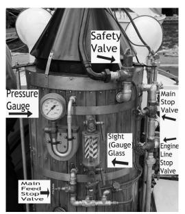
The following valves and equipment allow the addition and control of water level in the boiler:
