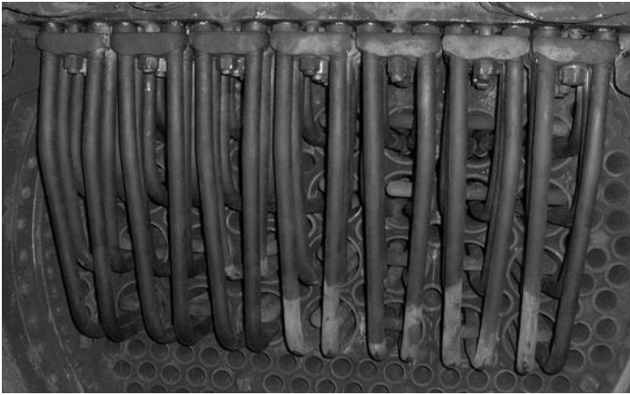
(left) A superheater header and superheater tubes on a steam locomotive
