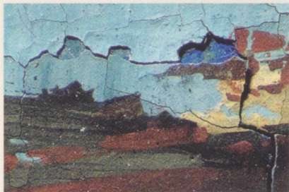
FIG.19 A CROSS-SECTION SHOWING THE NUMEROUS LAYERS OF OIL PAINT AND LARGER PIGMENT PARTICLES ADDED DRY BY THE ARTIST, SPANISH SHRINE
